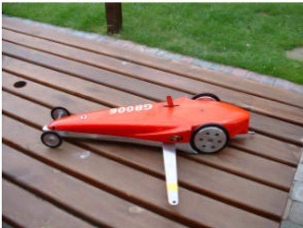
*The car at the start of the 2004 racing season. Re-modelled nose and tail areas are clearly seen in this view. Also to be noted in this picture is the alternative tether arm with yellow colour band. This allows the car to be run in the WMCR 3,5cc class.*
