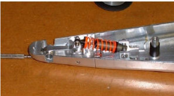
*Suspension assembly mounted in the nose of the car.*
