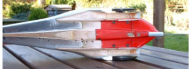
*View looking on the underside of the car showing the bypass channels, venturis and central airflow splitter.*
