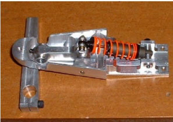
*The self-contained front suspension assembly, shown here minus front axle.*
