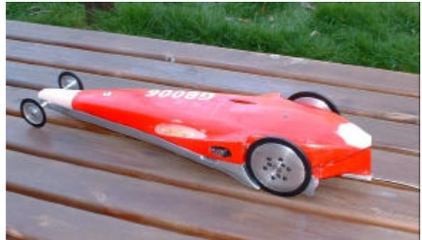
*View of the car after repairs to the tail and modifications to the nose to accommodate the lengthened wheelbase, prior to re-finishing. Balsa top covered with glass cloth and epoxy resin allows easy modification.*
