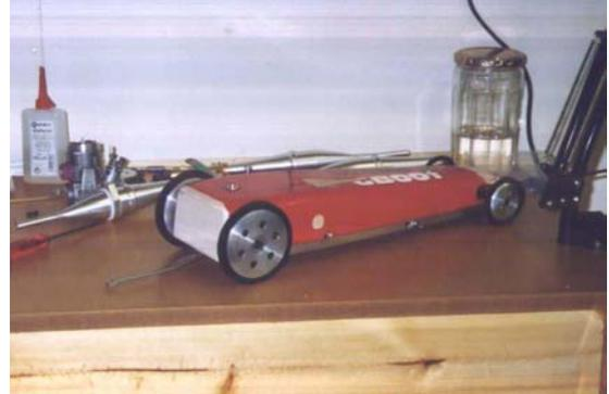
The car after surgery to the back end and prior to re-finishing with glass & epoxy.
