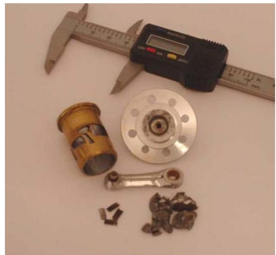
The internals of the motor – the pile to the right is the piston, the four small parts to the left are parts of the gudgeon pin. Damage to liner and cylinder head apparent in this view.
