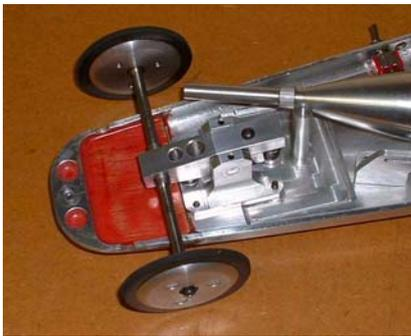
View of the front suspension with adjustable damping.
