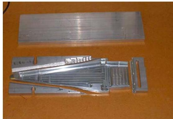
The fully machined lower pan, showing waste material and an unmachined blank. Total machining time approx. 30hrs.
